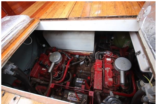
Gentleman's Yacht twin Beta engines and generator
