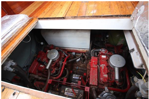
Gentleman's Yacht twin Beta engines and generator
